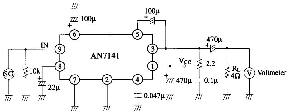
SG (Signal Generator) is seperated from pin 9 at measurement of Quiescent Current and Output Noise Voltage.
